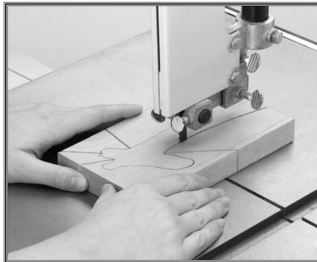
Figure 9. Use relief cuts for tight curves.
